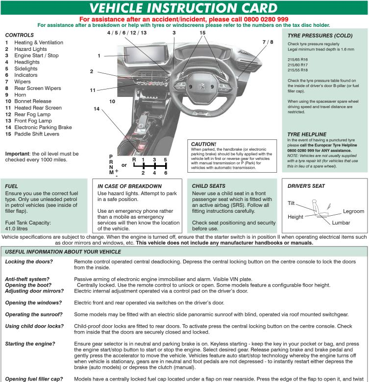
Pull bonnet release lever located on lower right hand side of front passenger footwell. Unhook catch under bonnet.
