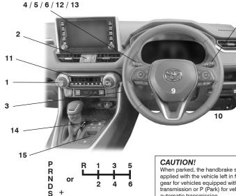
When parked, the handbrake should be fully applied with the vehicle left in first or reverse gear for vehicles equipped with manual transmission or P (Park) for vehicles with automatic transmission
